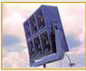
• **Long Range Focused Loudspeaker Array** is a ruggedized aluminum framework enclosing 6 directional horn loudspeakers. Array projects focused beams with spread of +/- 15° from center. Arrays can be stacked in two horizontal or vertical speaker sets and can be separated by up to 120 meters (400 feet). The unit works with UHF Tx/Rx set, and its rechargeable battery can be powered by 110/220VAC or 12VDC/24VDC.
